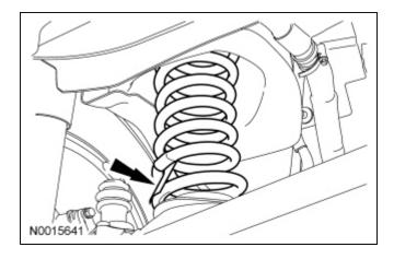
2. Raise the rear axle so the mark made on the rear shock absorber in Removal Step 1 lines up with the protective sleeve.
