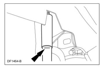
3. NOTICE: Tighten the shock absorber lower bolt while the suspension is at curb height or bushing damage and incorrect clamp load may occur.
